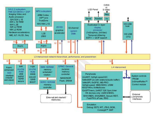
Figure 28. OMAP3530 Block Diagram
