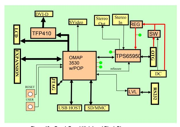
Figure 18. BeagleBoard High Level Block Diagram
