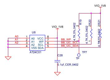
Figure 77. BeagleBoard Expansion Board EEPROM Schematic
