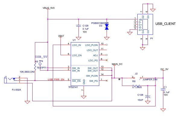
Figure 21. Input Power Section
