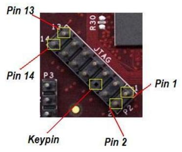
Figure 60. JTAG Connector Pinout
