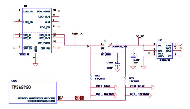
**Figure 22. Processor Current Measurement**
