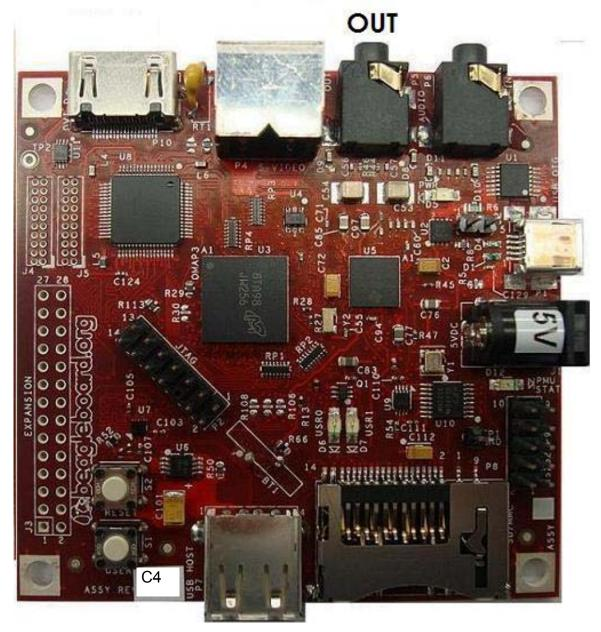
Figure 12. BeagleBoard Audio Out Cable Connection
