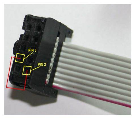
Figure 83. Serial Cable Loopback
