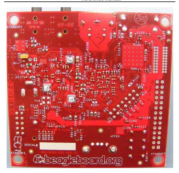
Figure 20. BeagleBoard Backside Components
