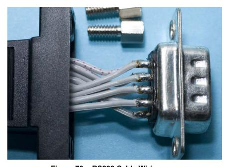
Figure 70. RS232 Cable Wiring
