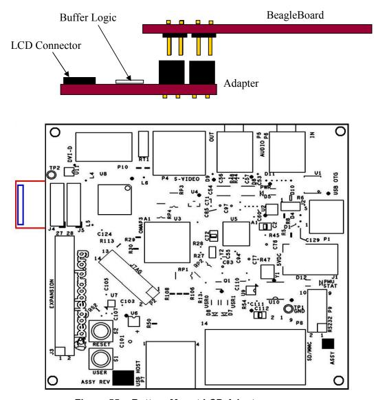
Figure 55. Bottom Mount LCD Adapter
