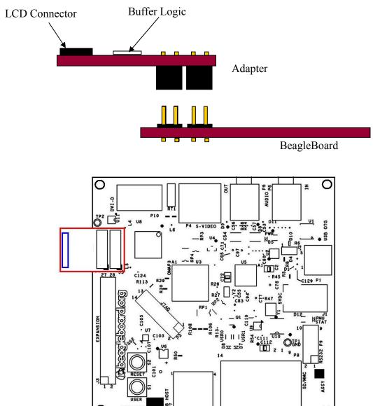
Figure 54. Top Mount LCD Adapter
