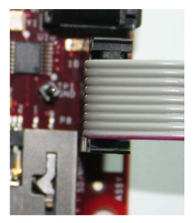
Figure 80. BeagleBoard Serial Cable Orientation
