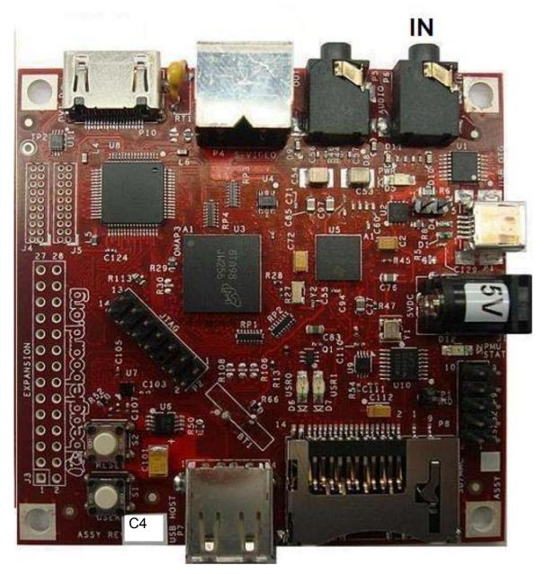
Figure 13. BeagleBoard Audio In Cable Connection
