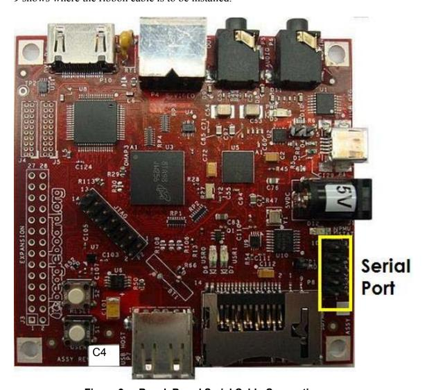
Figure 9. BeagleBoard Serial Cable Connection
